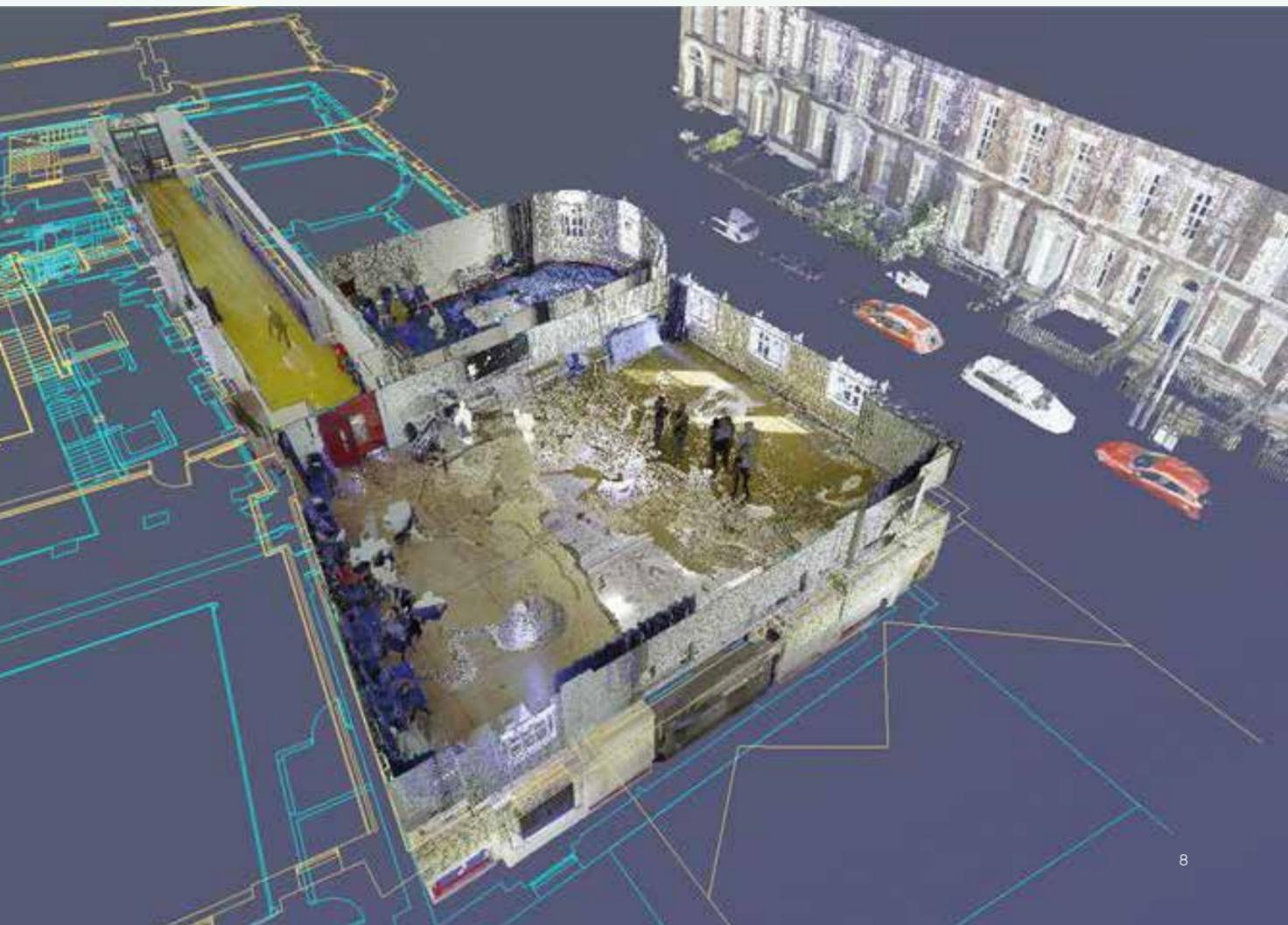
Ongoing work through LCR HOLISTIC expands on the previous collaboration and has introduced further digital techniques (such as photogrammetry and LiDAR) for capturing physical environments. The VEC team is working with MMA Design & Project Management and Auditive Limited to develop a powerful workflow for mapping the spatial audio characteristics of historic spaces and will carry out user evaluations to assess the effect of light, sound, and vibration in virtual twins.
